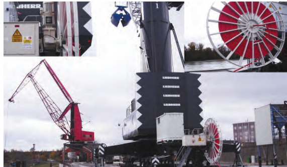
Mono spiral cable reeling drum on a large Liebherr mobile crane.
