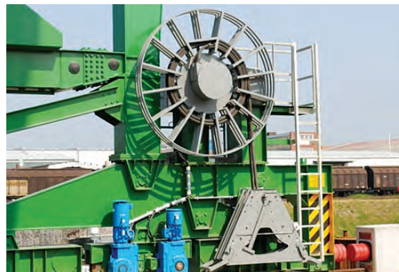
Twin cable spiral cable drum on large gantry crane.
