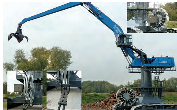
Large diameter double spiral motor driven cable reeling drum delivering twin power cables to a scrap handling crawler crane.
