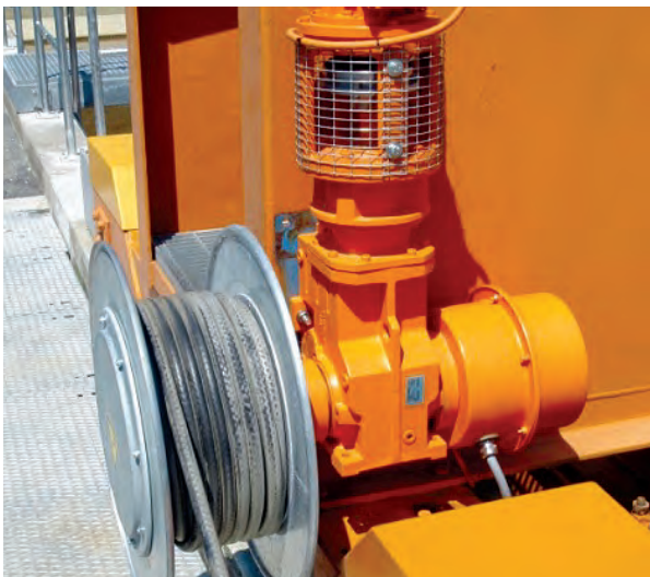
Twin cable spiral cable drum on large gantry crane.
